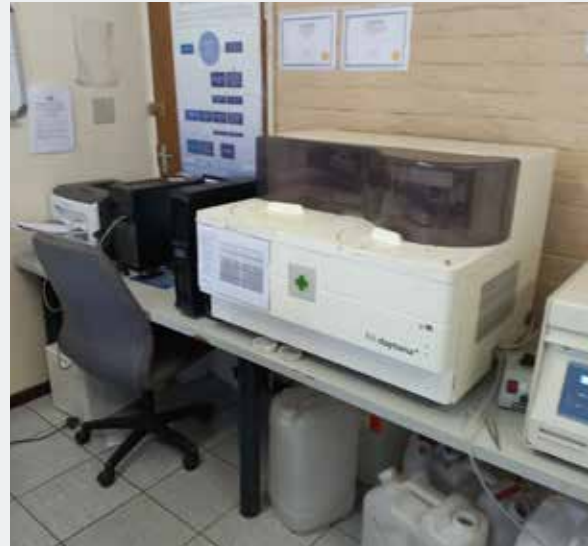
The RX Daytona is used for analyzing glucose, lipids, creatinine and various other tests.
