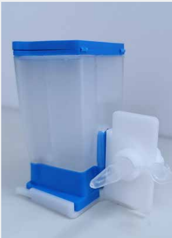
The CREDO device was designed by CTR members to extract useful material from used GeneXpert cartridges for downstream molecular tests, obviating the need for additional specimens, saving both the patient and healthcare system time and resources.
