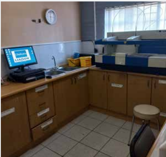
The DiaSorin analyser primarily used for Vitamin D analysis, also for other tests like insulin, Hep B and C-Peptide.
